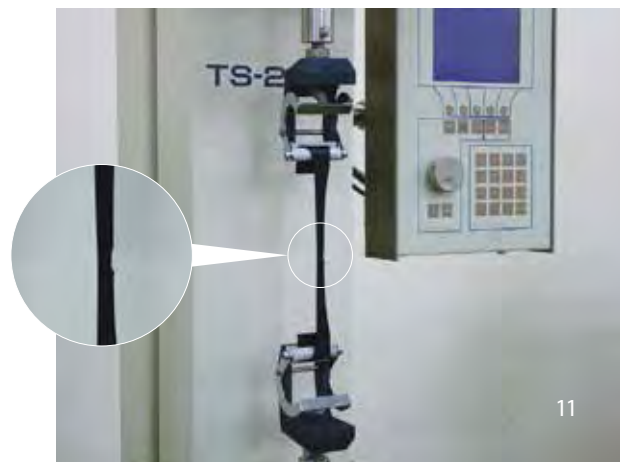
Tear strength test (crescent piece)
