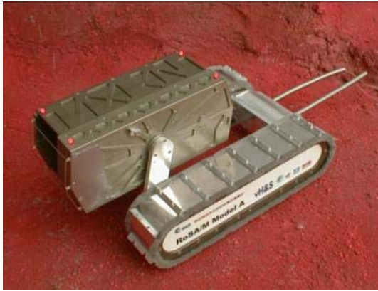
Figure 24: Nanokhod, developed by Hoerner and Sulger GMBH and the Max Planck Institute [22]
